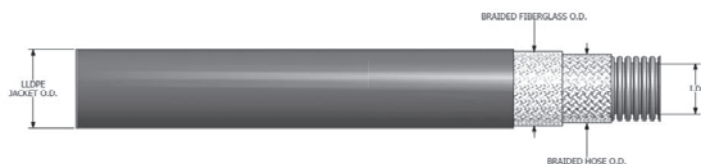
Figure 1 - Insulated Extruded Hose Dimensions
