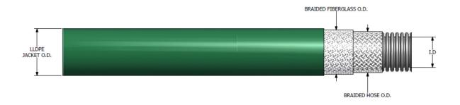
Figure 1 Insulated Extruded Hose Dimensions
